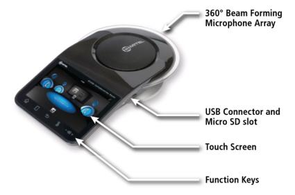
It has a patented beam forming microphone array that delivers 360° audio clarity for all participants. It automatically locates the talker in the room and attenuates background noise by adjusting the microphone sensitivity towards the current talker. It provides visual indication of the active speaker.
